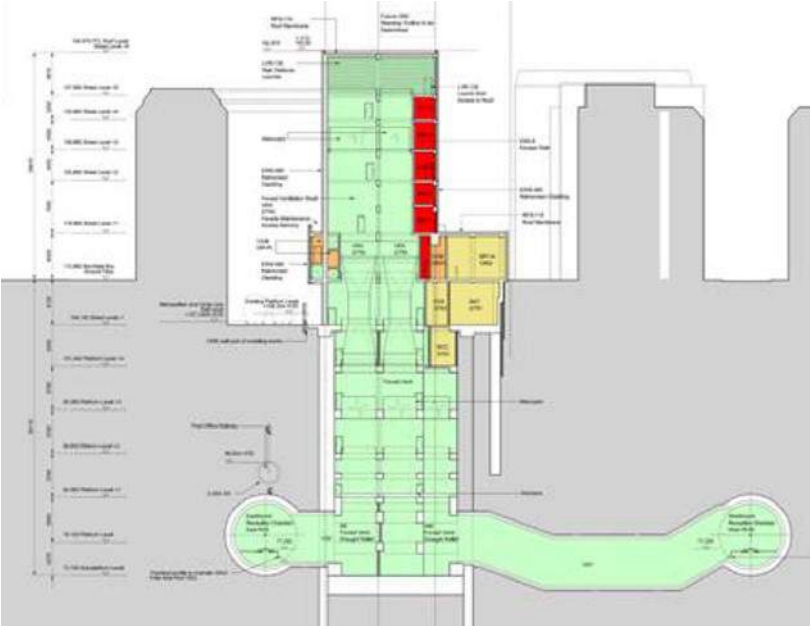
Fig.2. OSD and underground Metro station founded on compensated piled-raft.
